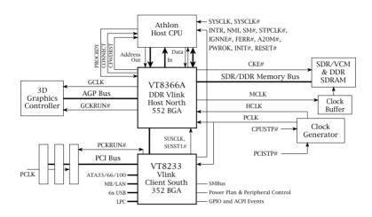
Diagram of Apollo Pro266A System Block Using the VT8233 V-Link South Bridge
