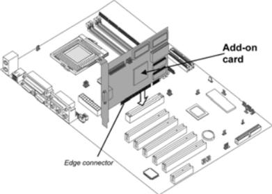
An isometric diagram of a computer motherboard showing an expansion slot. An add-on card is being inserted into the slot. A label 'Add-on card' points to the card, and a label 'Edge connector' points to the gold contacts on the card's edge. The diagram also shows other components like RAM modules and a cooling fan on the motherboard. |
