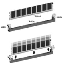
Install the DIMM module into the slot and press it firmly down until it seats correctly. The slot latches are levered upwards and latch on to the edges of the DIMM.
