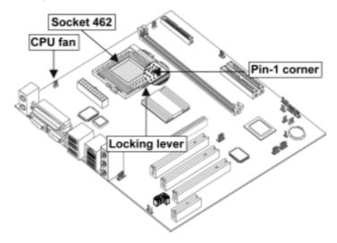
**Note:** The pin-1 corner is marked with an arrow
