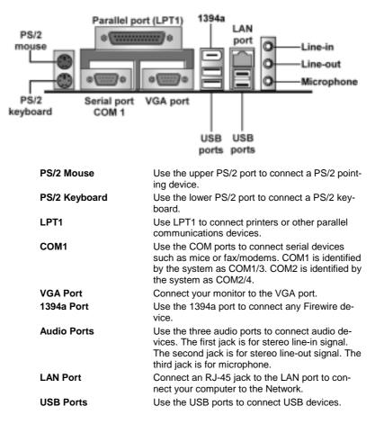
The backplane of the mainboard has the following I/O ports:
