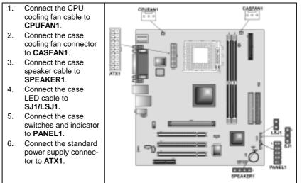
ATX1: ATX 20-pin Power Connector
