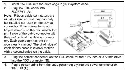
When you first start up your system, go immediately to the Setup Utility to configure the floppy diskette drives that you have installed. See Standard CMOS Feature on page 29 for more information.
