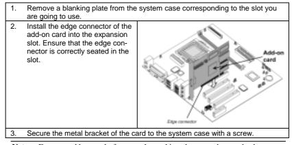
Note: For some add-on cards, for example graphics adapters and network adapters, you have to install drivers and software before you can begin using the add-on card.
