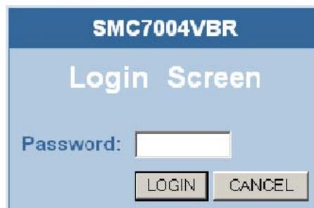
To log in to the management, enter the system default password “**smcadmin**” and click the **LOGIN** button. If you typed the password correctly, the left panel of the Web user interface changes to the administrator configuration mode as shown in the following figures.
