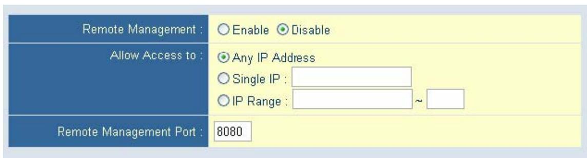
The screenshot shows the 'Remote Management' configuration section. It features three rows of settings: 1) 'Remote Management' with radio buttons for 'Enable' and 'Disable', where 'Disable' is selected. 2) 'Allow Access to' with radio buttons for 'Any IP Address', 'Single IP', and 'IP Range', where 'Any IP Address' is selected. The 'Single IP' and 'IP Range' options have corresponding input fields. 3) 'Remote Management Port' with a text input field containing the value '8080'.
