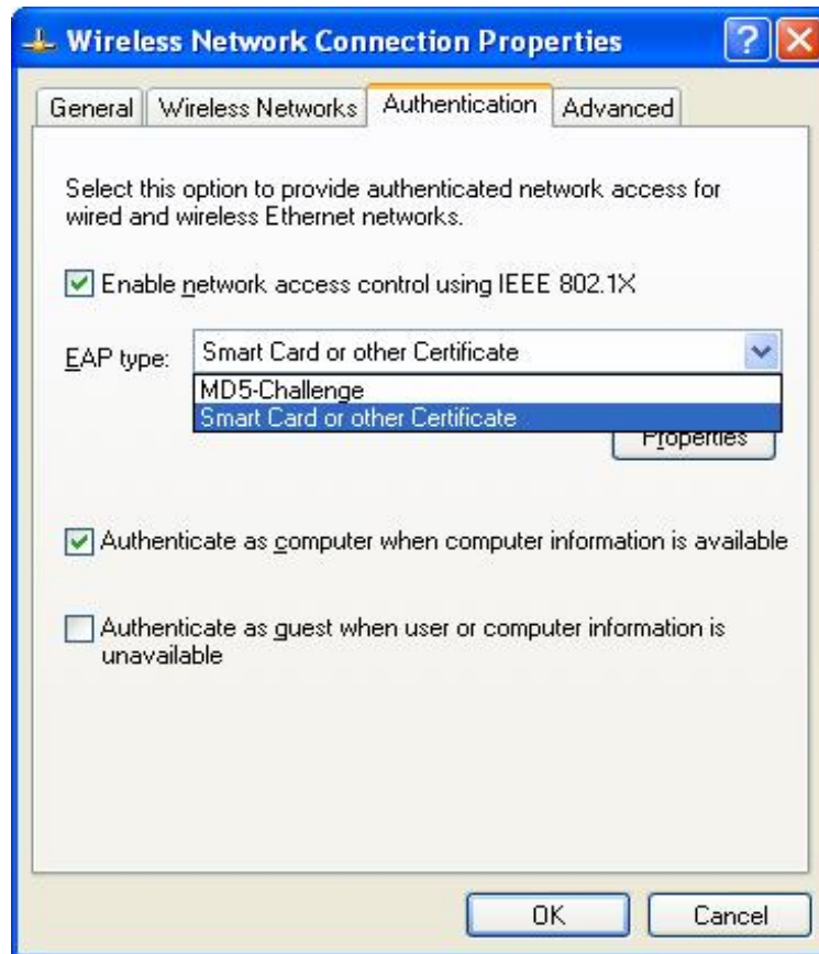
Figure 2: Enable IEEE 802.1X access control
